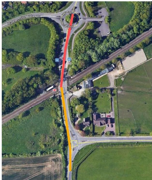
Plan 1: Extent of ramp required to "bridge" the railway line
